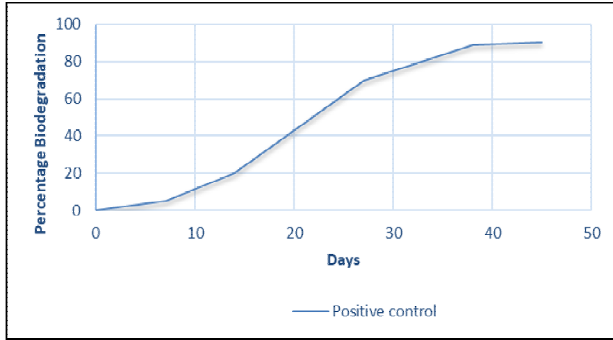
Graph-2a: The percent biodegradation of the Positive control (Reference material- Cellulose) determined based on conversion of carbon from cellulose to carbon in the gaseous phase ( \text{CH}_4 and \text{CO}_2 )
